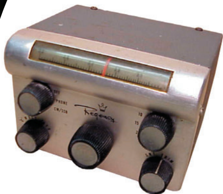
REGENCY MODEL ATC-1 - This amateur band converter was manufactured by the Regency division of I.D.E.A., Inc. of Indianapolis, IN. It operates on a transistorized circuit for reception of the 80, 40, and 20 meter bands, and can be used with any broadcast receiver, either automobile, portable or home receiver. ( Robert Enemark, Duxbury, MA )
