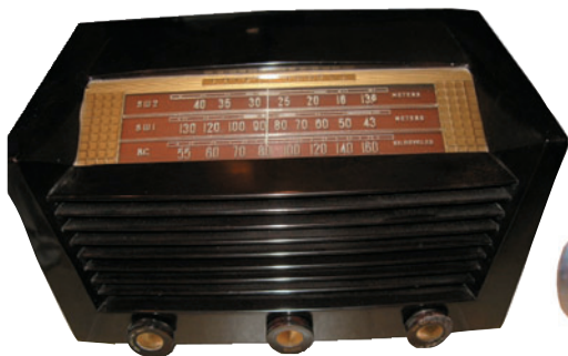
PHILCO TROPIC MODEL 3012 – This was made by Philco for the export market. It is unusual in that it has 3 bands: AM, SW1, and SW2. The 2 shortwave bands are marked in Meters instead of MC. ( Albert Johns, Phoenix, AZ )
