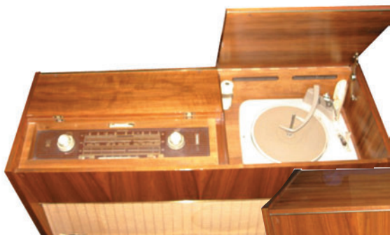
GRUNDIG MAJESTIC MODEL SO12U – Manufactured in 1959 by Grundig in Germany for the U.S. market. It has AM/FM and shortwave bands. The turntable was stereo but the radio was mono. (Andrew Bloor, Manhattan, KS)
