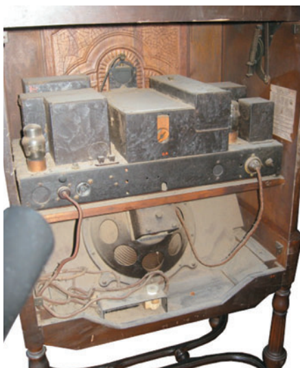
STROMBERG CARLSON MODEL 11A CONSOLE – Manufactured by Stromberg Carlson in 1930. The top lift up to reveal an optional turntable (missing from this example.) Very ornate wood with front doors. The chassis has 7 tubes including 2 #45 for the output. ( Jon Kummer, Port Washington, NY )
