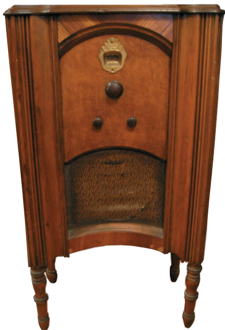
PHILCO MODEL 20 CONSOLE RADIO – Philco made this radio in 1930 in both the console and cathedral versions. This is a small console measuring 34" x 19" x 11". ( Robert Hughes, Lincoln, NE )
