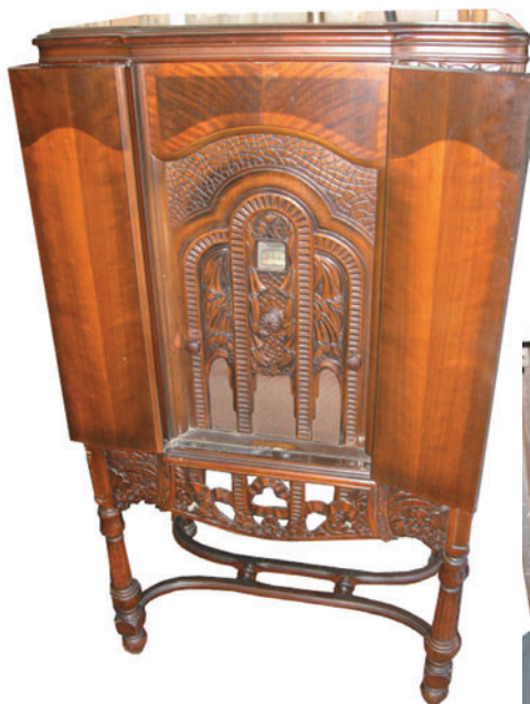
STROMBERG CARLSON MODEL 11A CONSOLE – Manufactured by Stromberg Carlson in 1930. The top lift up to reveal an optional turntable (missing from this example.) Very ornate wood with front doors. The chassis has 7 tubes including 2 #45 for the output. ( Jon Kummer, Port Washington, NY )
