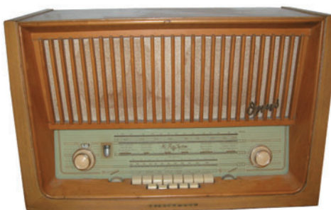
TELEFUNKEN OPUS 7 RADIO – Manufactured by Telefunken in Germany in 1956/1957. This blond version was made for the U.S. market. There were other Opus 7's made for the European market. Bands are AM, FM, Long Wave, and short wave. ( Elsa Kovey, Atlanta, GA )
