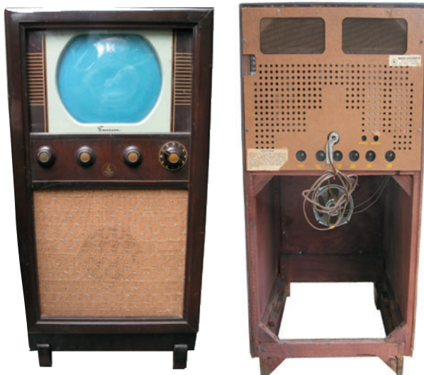
EMERSON MODEL 638 TELEVISION – Manufactured by the Emerson Radio & Phonograph Corporation in 1949. This television used a 10 inch CRT and a total of 22 tubes. The chassis was used in both table top and floor versions. ( Mark Arkin, Los Angeles, CA )
